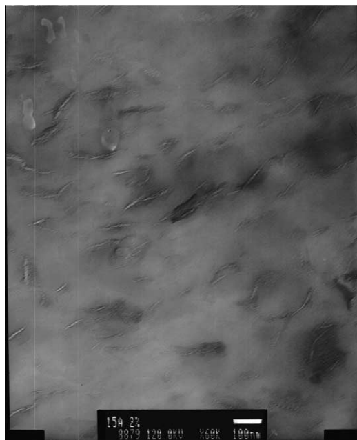
Fig. 5. TEM images of precipitated PVDF–nanoclay composite containing 2% 15A after hot-pressing into a film.
